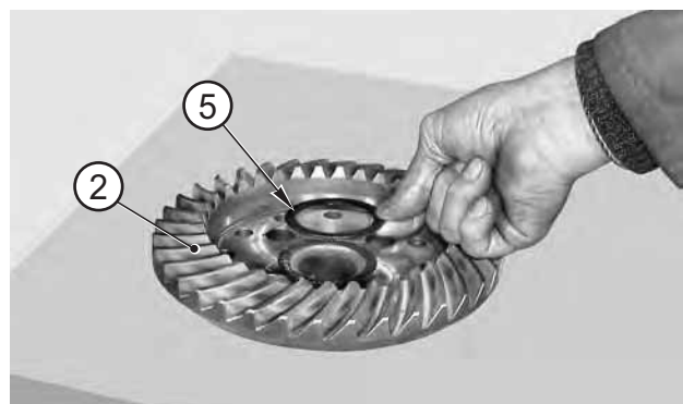
FIGURE 24: Position the shim washer (5) on the crown (2).
