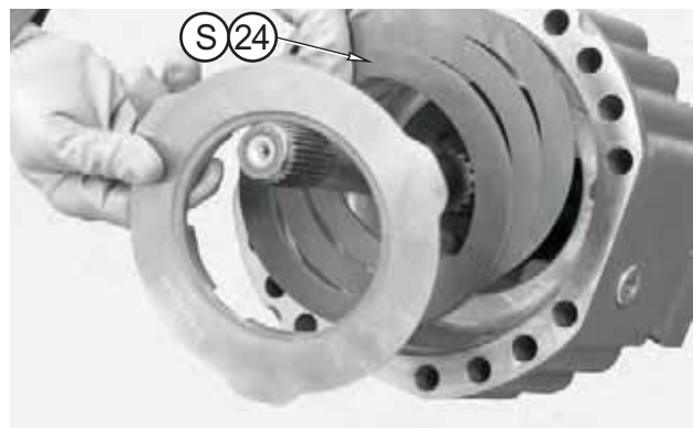
FIGURE 37: S = 68 \text{ mm} - (x + y + v) = Thickness of shims to insert under the shim washer.
