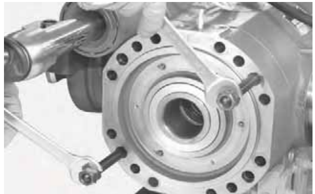
FIGURE 24: Lock the cylinder.
