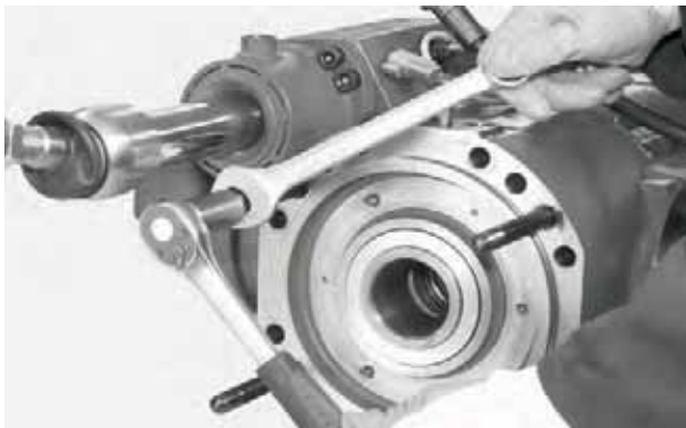
FIGURE 7: Loosen the studs and remove two of them.
