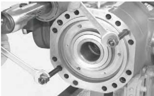
FIGURE 8: Loosen the studs and remove two of them.
