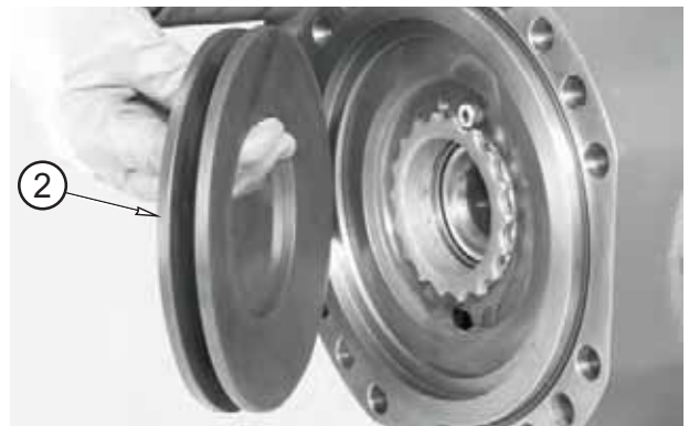
FIGURE 10: Remove the Belleville washers (2) and write down direction of assembly.
