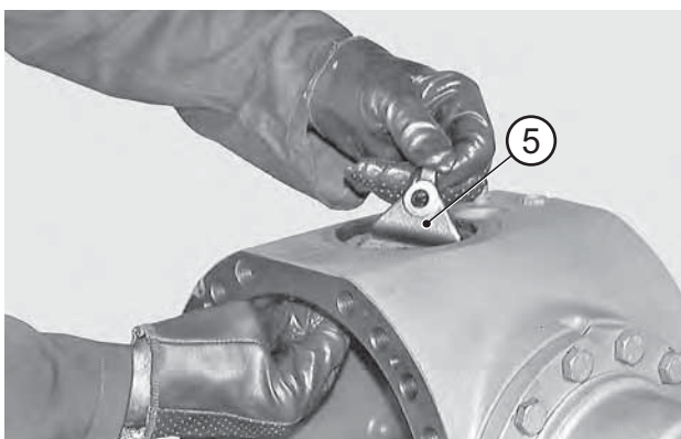
FIGURE 9: Extract selector fork (5).
