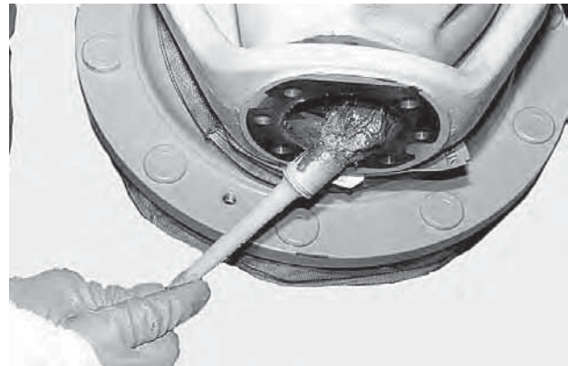
FIGURE 8: Lubricate steering case.
