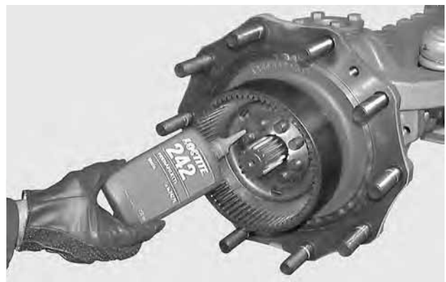
FIGURE 34: Apply Loctite 242 to the studs and fit on the nuts (4).
